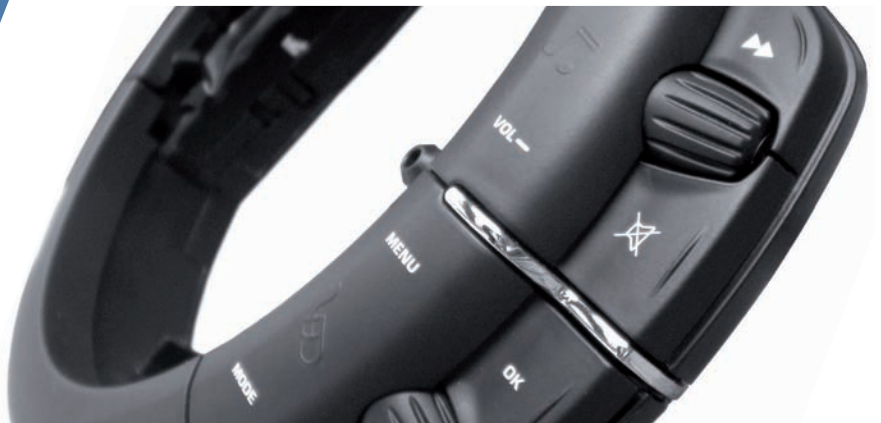
Cruise control buttons and LED light tracks, black paint on crystalline-PC base
